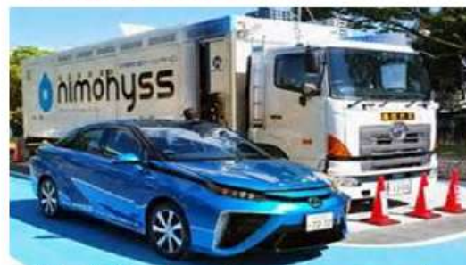
■ Mobile hydrogen station
